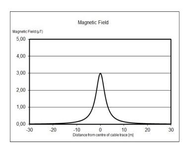
The magnetic field kept lower than  $0.4~\mu T$  in people's houses, in schools, in child day-cares, etc., measured in a height of 1.0 meter above ground.
